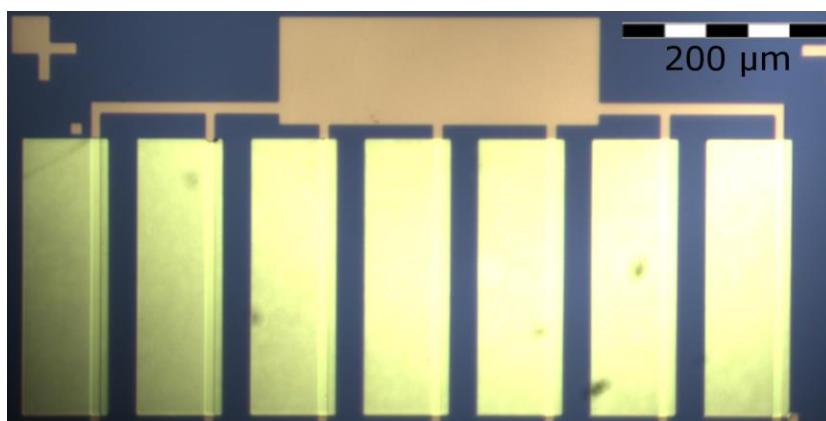
Figure S7. Optical microscope image of a typical final sample used for electrical measurements. The orange part is the grafted bottom electrodes, the yellow parts are top electrodes.
