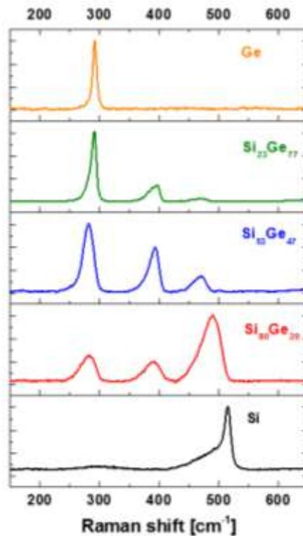
Figure 1: Raman spectra of the various  $\text{Si}_{100-x}\text{Ge}_x$  samples, from  $x=100$  (pure silicon) to  $x = 0$  (pure germanium).
