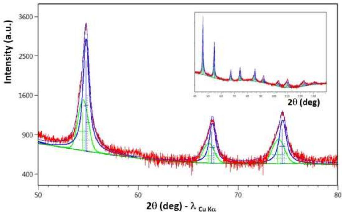
Figure 4 : X-ray diffraction peaks of  $\text{Si}_{53}\text{Ge}_{47}$  powder (red: experimental data – black: result of the Rietveld structure refinement considering two diamond-type crystalline phases to account for the chemical composition inhomogeneities – green and blue: contributions of the as determined  $\text{Si}_{0.35}\text{Ge}_{0.65}$  and  $\text{Si}_{0.5}\text{Ge}_{0.5}$  phases). The inset shows full experimental and refined diffractograms.
