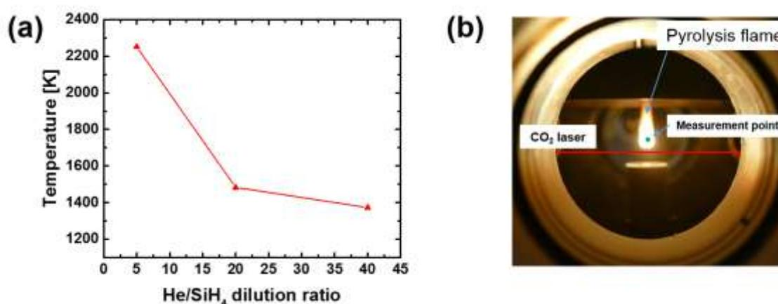
Figure 3: (a) Temperature measurement obtained by CARS spectroscopy during laser pyrolysis of Silane as a function of dilution rate (He/ $\text{SiH}_4$ ) and at 1050 W laser power (b) measurement points taken at 7 mm above the inlet
