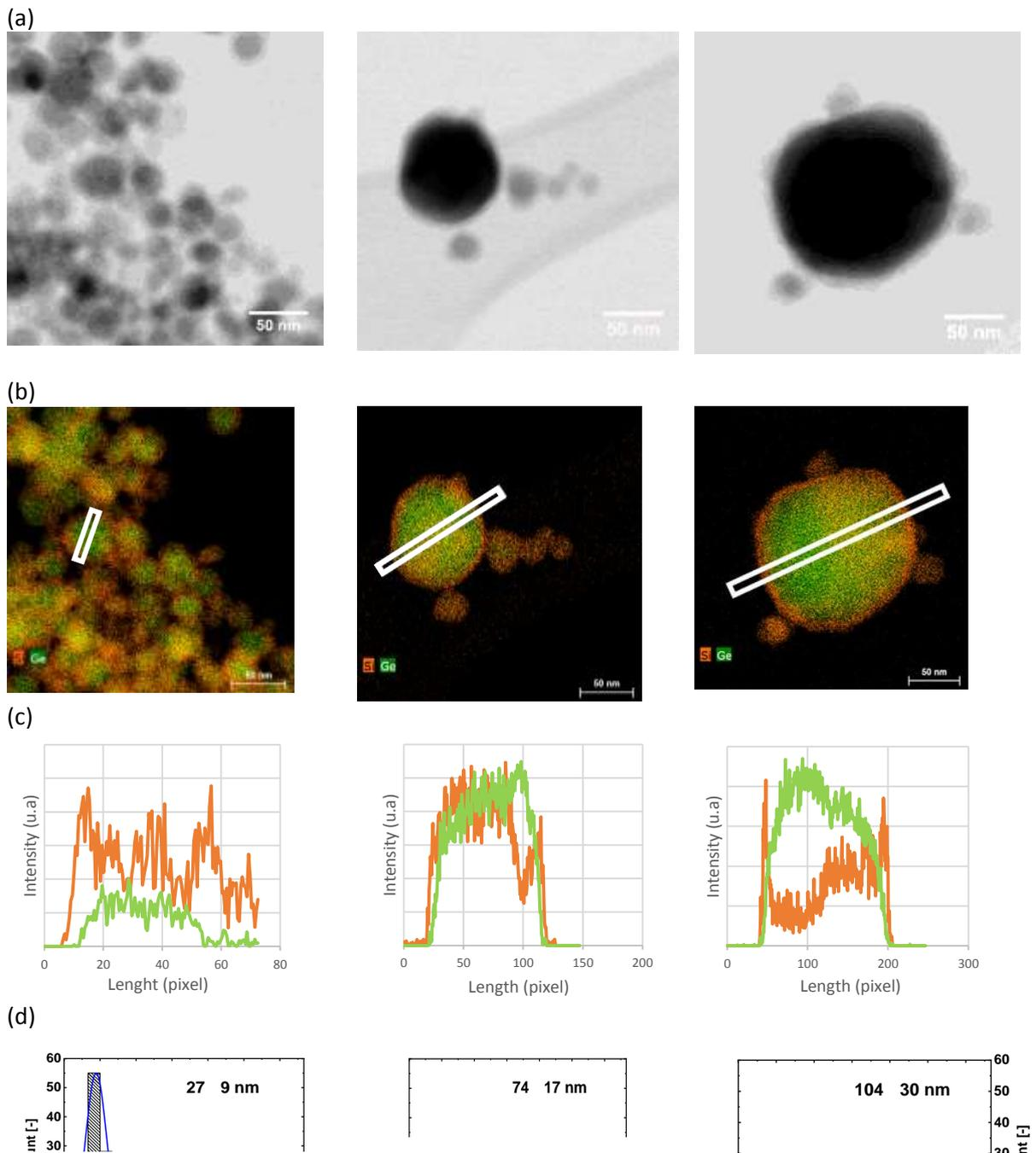
Figure 2 : a) STEM and b) STEM-EDX pictures of three Si<sub>100-x</sub>Ge<sub>x</sub> alloys: Si<sub>80</sub>Ge<sub>20</sub> (left column), Si<sub>53</sub>Ge<sub>47</sub> (middle column) and Si<sub>23</sub>Ge<sub>77</sub> (right column), green color corresponds to Ge atoms while orange color corresponds to silicon. The white box on the STEM-EDX pictures corresponds to the position where EDX profiles are obtained as plotted in (c). c) Silicon (orange color) and Ge (green color)
