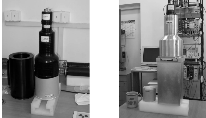
Figure 10. Large volume NaI(Tl) detectors purchased for the EURITRACK project: 5"×5" (left) and 5"×5"×10" (right) crystals, both with XP4512B PMT.
