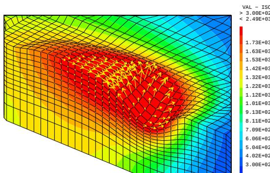
**Figure 4.** Calculated weld pool with considering free surface.
