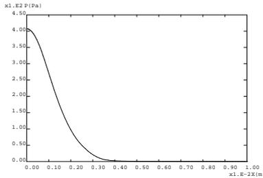
**Figure 1.** Radial evolution of arc pressure [7].
