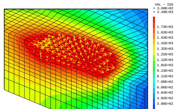
**Figure 5.** Calculated weld pool without considering free surface.
