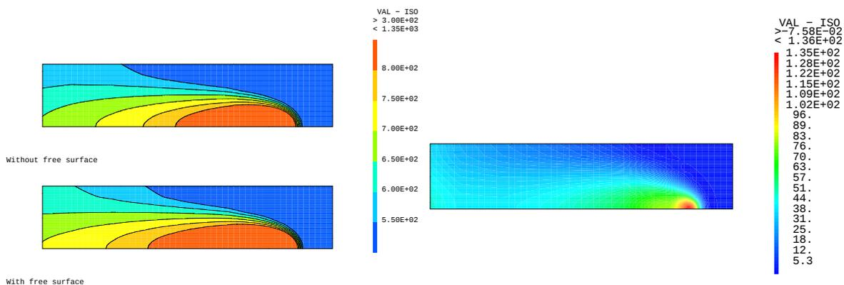
**Figure 6.** Calculated temperature field at the bottom surface of workpiece for the case without and with considering free surface.
