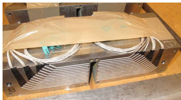
Fig. 2 Thermocouple location at one block surface
