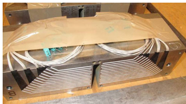
Fig. 2 Thermocouple location at one block surface
