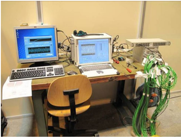
Fig. 3 Temperature, amperage, and voltage acquisition setup
