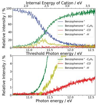
**Fig. 7** Breakdown diagrams of the benzophenone cation fragmentation, built from the SPESs of Fig. 3 (top panel) and from the total ion yield of Fig. 4 (bottom panel). The full scale of this last graph is presented in the ESI.† These diagrams are relative and show the passage from parents to fragments.<sup>43,44</sup>
