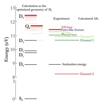
**Fig. 8** Energetics of the benzophenone molecule and cation, summarizing calculations and experimental data. The thin red lines simulate Rydberg series (quantum defect  $\delta$  = 0.1) converging towards the D<sub>4</sub> and Q<sub>0</sub> states of the cation. For the fragmentation processes in action, see the text.
