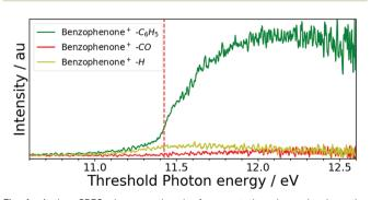
Fig. 4 Action-SPESs documenting the fragmentation channels where the benzophenone ion has lost either a  $C_6H_5$  (green curve), a CO (red) or a H (dark yellow) group. The SPESs were constructed by considering the photoelectron energies in the range 0–1.4 eV when projecting the SPES-matrix. The vertical dash red line at 11.421 eV indicates the steep increase observed in the full blue curve in Fig. 3.
