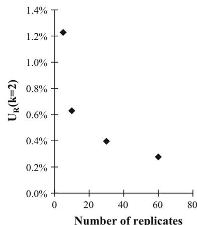
**Fig. 2** Evolution of the ratio expanded uncertainty with the number of replicates. [Zr] = 10 μg L<sup>-1</sup> and [Mo] = 10 μg L<sup>-1</sup> in the dilution matrix
