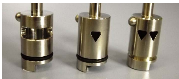
Fig. 4. Aqueous weir, from left to right: original (a), first improvement (b), final shape (c).
