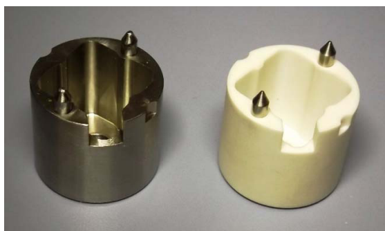
Fig. 2. Mixing chamber (stainless steel and PTFE).
