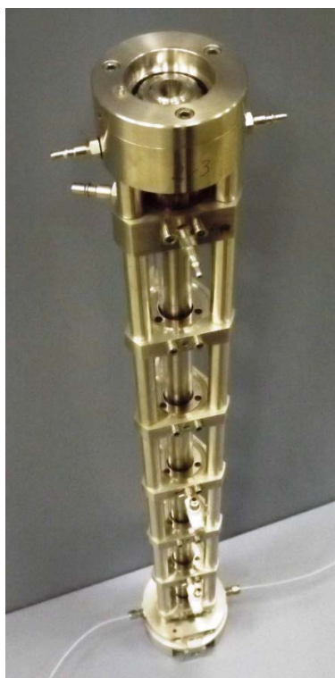
Fig. 6. Taylor-Couette column designed for use in hot cells.
