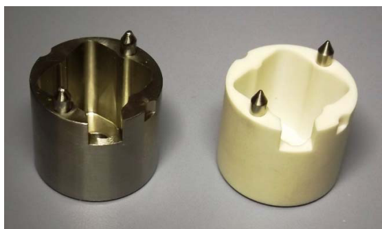
Fig. 2. Mixing chamber (stainless steel and PTFE).
