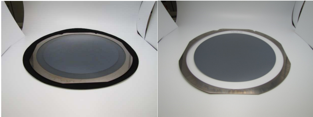
Figure 10: Pictures of the 70 \mu\text{m} wafer mounted onto a frame (left: before cleaning the adhesive and right: after cleaning the adhesive)
