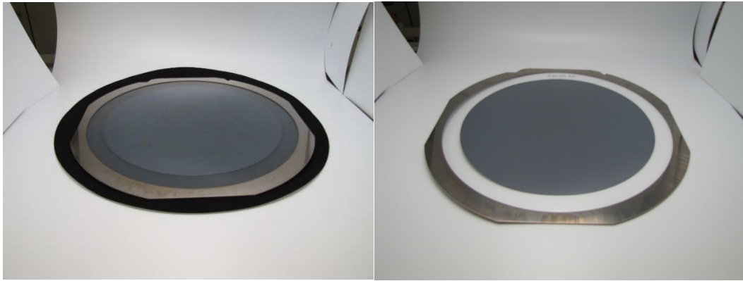
Figure 10: Pictures of the 70 \mu\text{m} wafer mounted onto a frame (left: before cleaning the adhesive and right: after cleaning the adhesive)
