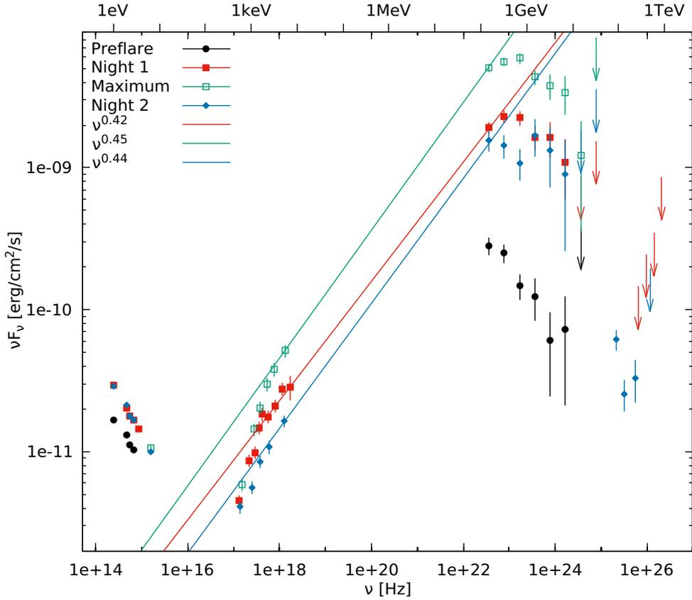
**Fig. 4.** Observed multiwavelength SED for the considered time frames with black dots for the Preflare time frame, red filled squares for Night 1, green open squares for the Maximum, and blue diamonds for Night 2. The  $\gamma$ -ray data have been corrected for EBL absorption using the model by Franceschini et al. (2008). The solid lines show a power-law interpolation for the X-ray to  $\gamma$ -ray spectrum, as described in the text.
