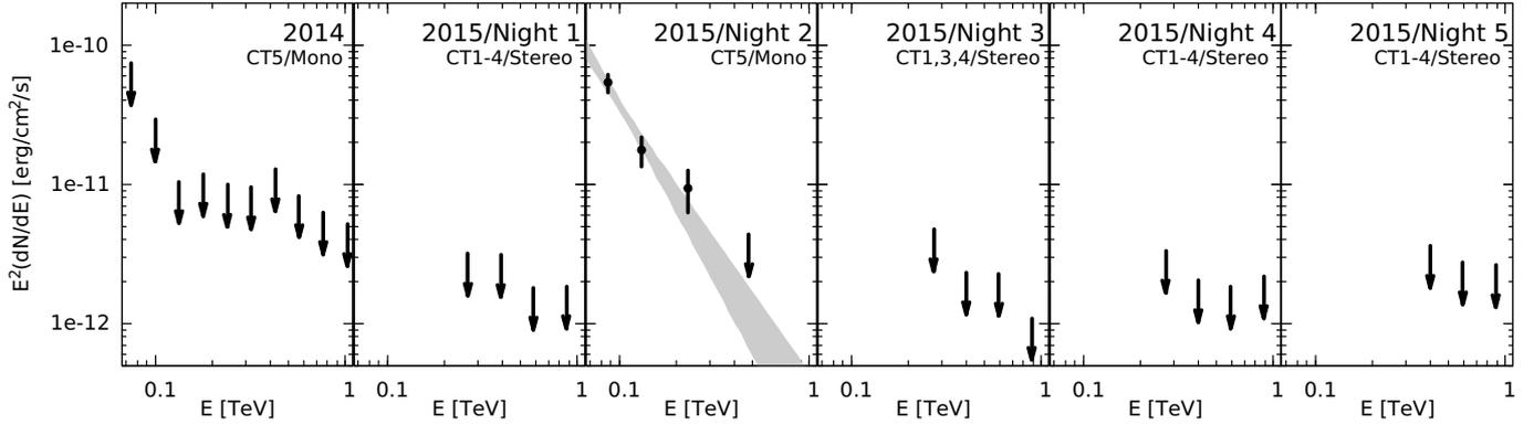
**Fig. 1.** Observed H.E.S.S. photon spectra for six data sets as labeled. Arrows mark upper limits (99% confidence level). The gray butterfly is the  $1\sigma$  statistical uncertainty band of the 2015/Night 2 data set. Error bars are statistical only. The second label gives the telescope participation and the analysis used.
