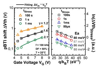
Figure 11. Voltage acceleration factor evaluation under AC stress (left) and activation energy extraction (right) extracted on MOSc-HEMT technology. Frequency is set at 100kHz to be close to operating conditions.
