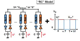
Figure 8. Schematic of the RC network used BTI modeling [13,15]. Each traps is represented by a combination of a capacitor C and by two resistances Re and Rc to set emission and capture time respectively. In the case of AC BTI, this circuit is studied under a Vg signal given by the chronogram (right) which gives access at the capacitor voltage U(t) after a given number of cycles.
