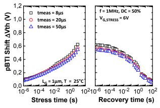
Figure 4. AC pBTI stress and recovery characteristics as a function of the  $I_D(V_G)$  measurement time.  $L_G=1\mu m$  and  $T=25^{\circ}C$  for this measurement.
