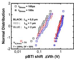
Figure 14.  $\Delta V$ th distributions after two stress times (100 $\mu$ s and 100s). No visible difference is observed between 0.5 and 1 $\mu$ m gate length. f = 1MHz and  $V_{G,Stress}$  = 7V here.
