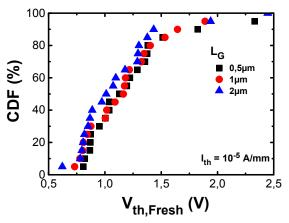
Figure 2. Cumulative distribution function of Vth for different  $L_G$  (0.5, 1 and  $2\mu m$ ) confirming the E-mode operation (Vth > 0V). Drain voltage is set at  $V_D = 0.1 V$ .
