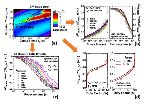
Figure 9. (a) Capture and Emission Time (CET) map giving the traps density  $g(\tau c, \tau e)$ . This map shows two population, one for short time degradation and a second one for long time degradation with a very specific emission time around 4-5s. Comparison of experimental and modeled  $\Delta V$ th (b) stress and recovery for increasing frequencies, (c)  $\Delta V$ th recovery after increasing AC stress time (1ms to 1ks) and (d)  $\Delta V$ th AC/DC degradation ratio as a function of DF.
