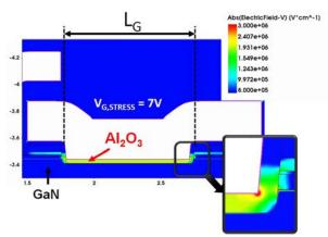
Figure 10. TCAD simulation of electric field distribution under  $V_{G,Stress}$  = 7V on 30nm Al<sub>2</sub>O<sub>3</sub>/GaN MOS gate stack including gate field plate and GaN-UID recess introduced in section II-A. Gate length is set at  $L_G = 1 \mu m$  here. Whiteout areas are related to metalic materials.
