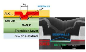
Figure 1. Schematic of the GaN-on-Si E-mode MOSc-HEMT gate stack and TEM cross section of a 0.5  $\mu$ m long recessed gate.
