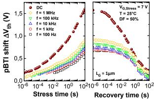
Figure 5. AC pBTI stress and recovery characteristics as a function of the signal frequency at DF = 50%. Filled symbols represent the DC pBTI case.  $L_{\rm G}$  = 1 $\mu m$  and T = 25°C for this measurement.the stress.
