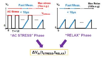
Figure 3. Principle of the AC pBTI measurement with ultra-fast Vth measurements minimizing unwanted Vth relaxation during the stress.
