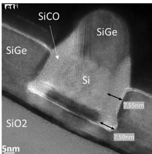
FIG. 11. TEM view after SiCO spacer etching using H_2 plasma (400 V) followed by a 210 s 1% HF dip and SiGe epitaxial growth.
