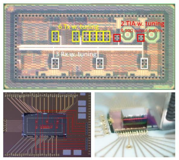
Figure 7: Die photographs of CMOS Transceiver chip with 6 Tx'es and 5 Rx'es including ring tuning, associated flip-chip face-to-face assembly on Si-photonic chip, and board & fiber integration
