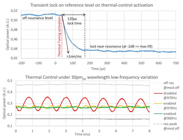
Figure 5: Transient thermal control behavior showing heater lock on target power level after activation and steady state tracking under environmental variation, here laser wavelength
