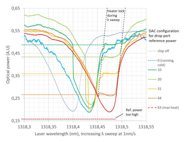
Figure 4: Thru-port transmission spectrum of a microring with different thermal tuning configurations, showing the heater locked (on Drop port) to a reference level during wavelength sweep
