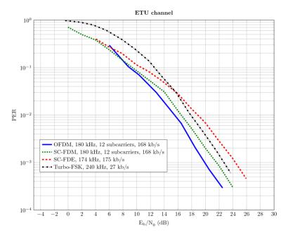
Fig. 1. PER as the function of the Eb/No for OFDM, SC-FDM, SC-FDE and Turbo-FSK.
