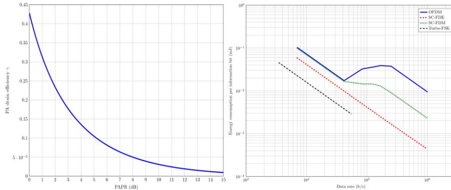
**Fig. 3.** (a) PA drain efficiency as a function of the PAPR (left).
