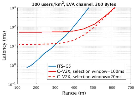
Fig. 8. ITS-G5 and C-V2X latency as the function of the range for a density 100 users/km<sup>2</sup>.
