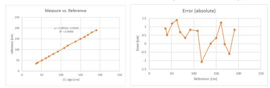
Figure 4: Distance detection of the Ultrasound module
