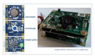
Figure 5: Long range LiDAR module (optic board on top of mother board)
