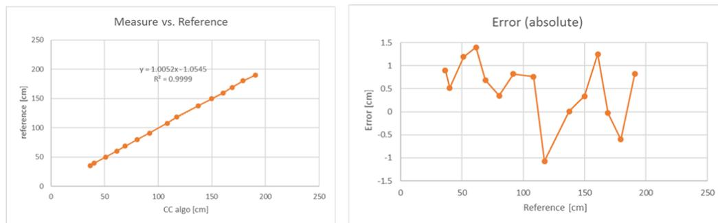
Figure 4: Distance detection of the Ultrasound module
