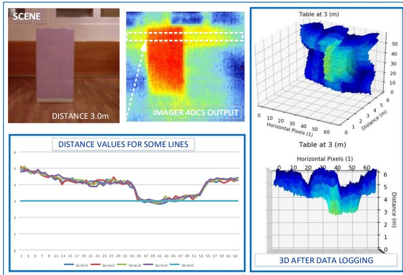
Figure 7: set-up image captures, distance measurement capabilities
