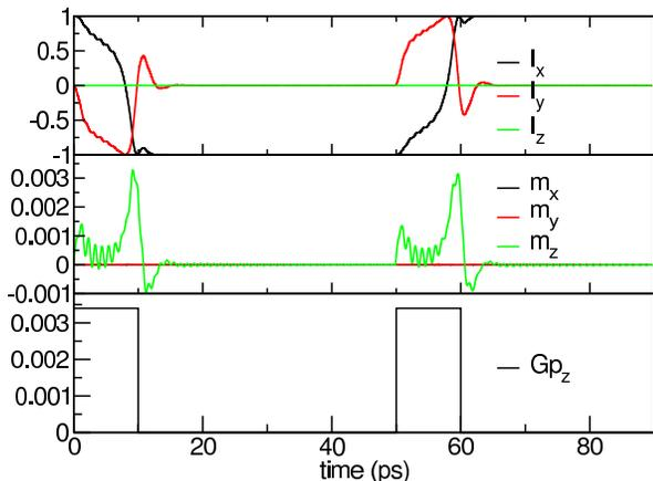
Figure 3. (Color online) Average magnetization (upper panel) and Néel order parameter components (middle panel) for a coupled switching with parameters in reference<sup>22</sup>. The lower panel displays the STT pulses. Here  $B_0 = 7.7\mu_0 M_s^2$  and  $B_1 = -23\mu_0 M_s^2$ .
