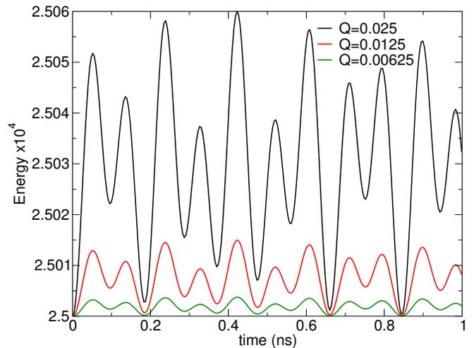
Figure 5. (Color online) Single-site total energy as a function of both time and variable timestep  $Q$ . Conditions of the simulation are expressed in reduced units:  $2C_0/\mu_0 M_s^2 = 5.1 \times 10^5$ ,  $2C_1/\mu_0 M_s^2 = 3.5 \times 10^5$ ,  $M_1 V_0 \mu_0 M_s^2 / 2\hbar^2 = 1000$ ,  $\omega_{DC} = (0, 0, 2\pi)$  rad.GHZ,  $\pi_{11}(0) = 1$ ,  $\mathbf{s}(0) = (1, 0, 0)$ . All the other parameters not reported, included initial conditions are zero.
