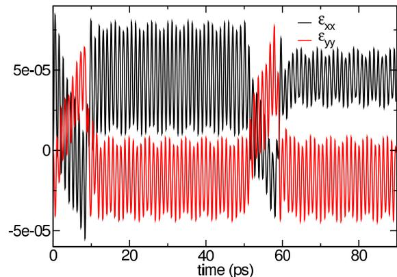
Figure 4. (Color online) Strain components as a function of time with the magnetoelastic constants turned on with parameters in reference<sup>22</sup>.
