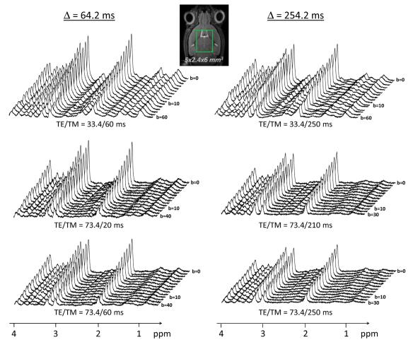
FIG. 4. Typical stack plots of spectra acquired for each TE/TM combination for the two different diffusion times. Each stack plot shown here is acquired in a single experimental session, in a large  $5 \times 2.4 \times 6$  mm<sup>3</sup> voxel in the mouse brain. For simplicity the lowest *b*-value was noted "b = 0", while it is actually slightly higher (see text for details). Note the excellent SNR (no line broadening was applied).
