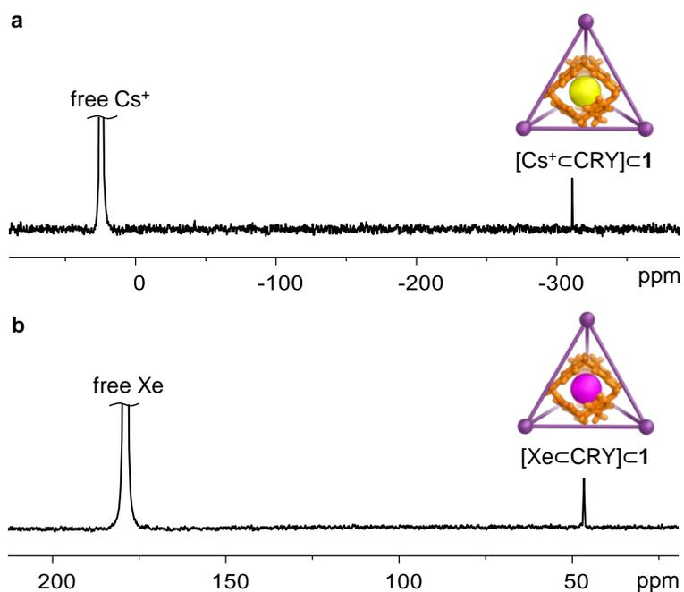
**Figure 3.** (a)  $^{133}\text{Cs}$  NMR ( $\text{CD}_3\text{CN}$ , 66 MHz, 60 °C) spectrum of CRY $\subset \mathbf{1}$  in the presence of excess  $\text{Cs}^+$ . (b)  $^{129}\text{Xe}$  NMR ( $\text{CD}_3\text{CN}$ , 138 MHz, 25 °C) spectrum of CRY $\subset \mathbf{1}$  in the presence of excess Xe.
