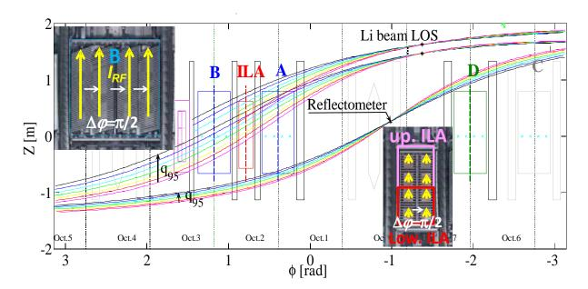
Figure 1: Toroidal/vertical view of ICRF antennas and outer limiters in JET from inside the vacuum vessel. Magnetic field line tracing from several points along Lithium beam and reflectometry LOS on pulse JPN 90454, over a scan of  $q_{95}$ . Inset: photos of A2 and ITER-like ICRF antennas, with sketch of the toroidal phasing.
