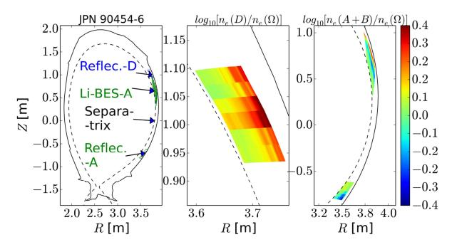
Figure 3: 2D maps of  $n_e$  ratios during antenna D and A+B to ohmic, mapped to antennas D and A.
