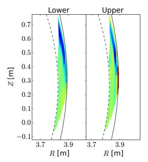
Figure 4 compares  $n_e$  modifications when powering lower and upper ILA, along the Li-beam LOS connected magnetically to the upper array.  $n_e$  changes in this region even when the un-connected lower ILA is active. When switching to the upper array, the density depletion stays similar in the upper part of the map while an over-density area develops at the bottom.
