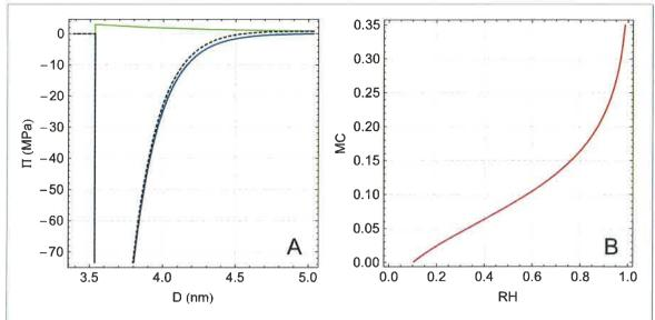
Figure 2. Contact points and hydration force contributions to the free energy changes. (A) Osmotic pressure II versus cellulose crystals center to center separation. Light green and blue curves represent H-Bond and hydration force contributions respectively. The dashed black curve is the sum of the two. (B) Resulting sorption isotherm.
