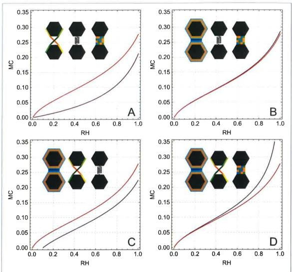
**Figure 5.** Contribution of each term to the total force balance. Sorption isotherms calculated considering all the terms in the force balance (red curves) or selectively excluding one (purple curves) of the following: (A) hydration repulsion, (B) contact points, (C) mixing entropy and (D) elastic energy.
