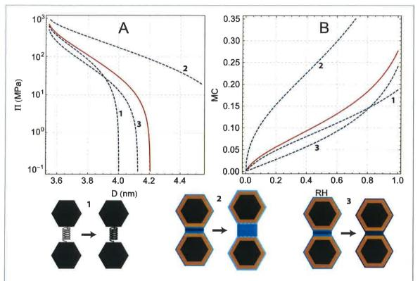
Figure B1. Changes in wood EOS as a results of chemical treatments. (1) Cross-linking (increase in matrix modulus). (2) Processing in highly basic solutions (charging of matrix polymers and cellulose surfaces). (3) Hydrophobization of matrix polymers (reduced hydration repulsion) (A) Moisture content versus relative humidity. (B) Osmotic pressure versus cellulose crystals center to center separation. The red curve represents the calculated EOS of the untreated wood tissue.
