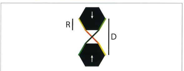
Figure A2. Matrix polymers bridging cellulose crystals. The portion of polymers (green for lignin and orange for hemicelluloses) contacting the crystals are depicted in brighter colours.
