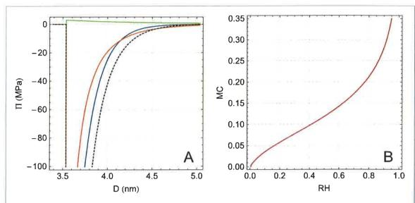
Figure 3. Configurational entropy contribution to the free energy changes. (A) Osmotic pressure  $\Pi$  versus cellulose crystals center to center separation. The orange curve represents the configurational entropy contribution while the dashed black curve is the sum of H-bond and hydration force (respectively light green and blue). (B) sorption isotherm resulting from the sum of the three contributions.
