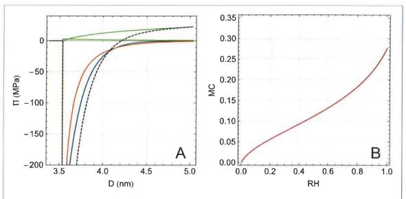
Figure 4. Total force balance. (A) Osmotic pressure  $\Pi$  versus cellulose crystals centre to centre separation. To the total force (black dashed curve) the following terms contribute: light green for the contact points term; blue for hydration force, orange for the configurational entropy and dark green for the elastic energy. (B) Sorption isotherm calculating from the sum of all the terms.
