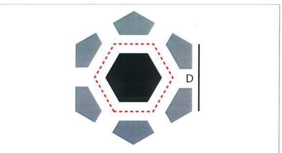
Figure A1. Unit cell (red dashed line) used for the force balance. The black hexagons represent the cellulose crystals. D is the center-to-center separation between them.
