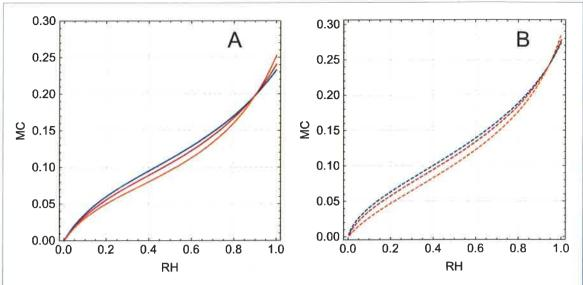
Figure 7. Comparison between (A) the experimental (from [42], desorption branch) sorption isotherms at different temperatures and (B) the sorption behavior predicted by the model (dashed lines). Blue: 14 °C, red, 24 °C, orange: 43 °C.
