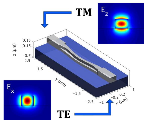
Fig. 1. Schematic of a two-level photonic polarization rotator.
