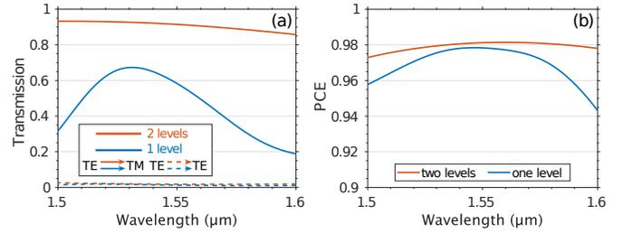
**Fig. 4.** Comparison of both transmission (a) and polarization conversion efficiency (b) between the one and two levels  $4 \mu\text{m}$  length designs.
