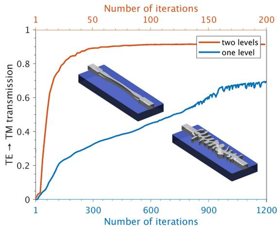
**Fig. 3.** Convergence graph of the figure of merit for the one and two levels  $4 \mu\text{m}$  polarization rotators (notice the two different  $x$ -axis). One iteration corresponds to  $\sim 10$  minutes of computation using a 20 cores 3 Ghz CPU.
