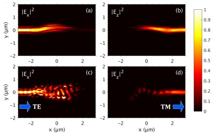
**Fig. 2.** Slice of the electric field at  $z = 0$  showing polarization rotation. (a),(b) two-levels design (c),(d) one-level design. FDTD (Finite Difference Time Domain) simulations at  $\lambda = 1.55 \mu\text{m}$ .
