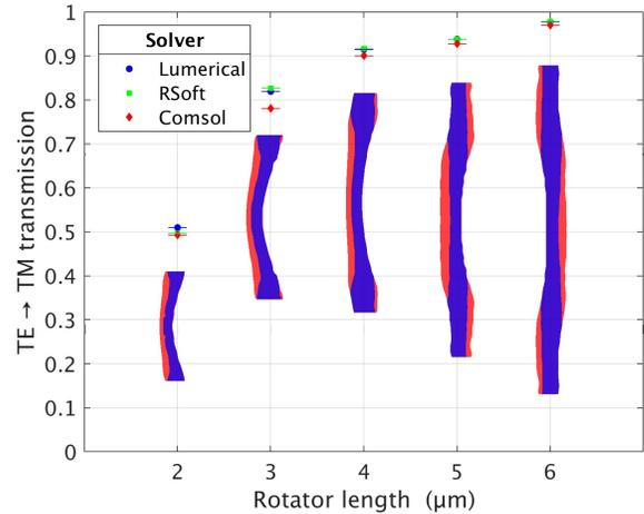
**Fig. 5.** Transmission of two-levels polarization rotators from  $2 \mu\text{m}$  to  $6 \mu\text{m}$  in length. Each device is represented in red (bottom level) and blue (top level).
