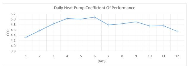
Fig. 14: Daily Heat pump coefficient of performance
