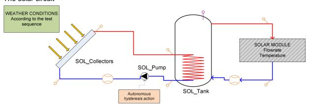
Fig. 4: Hydraulic diagram of the virtual solar circuit
