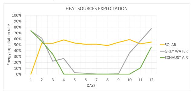
Fig. 11: Evolution of the exploitation rate of each heat source during the test sequence
