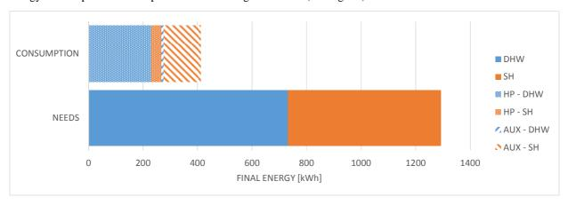
Fig. 15: Comparison between the heating needs and the final energy that would be consumed by the heat pump and the theoretical external auxiliary systems
