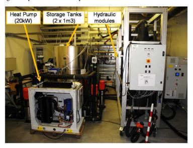
Fig. 2: Pictures of the system tested on the semi virtual test bench
