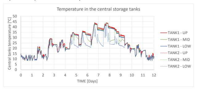
Fig. 12: Evolution of the temperatures measured in the central storage tanks during the test sequence
