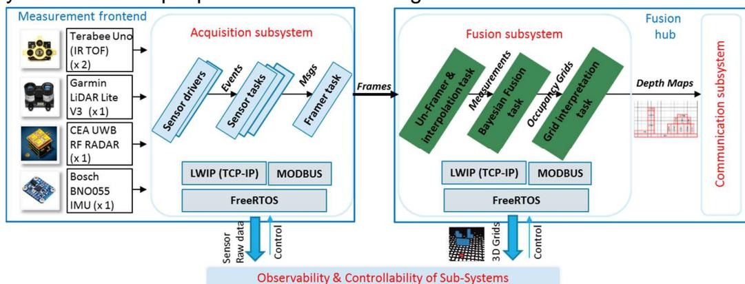
Fig. 4: first prototype overview (mobile detection device)
