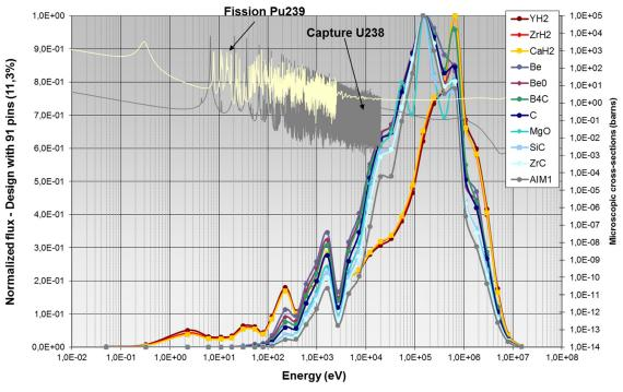
Fig. 2. Neutron spectra for different types of neutron moderator materials in the core (11% in volume fraction) compared with a reference case without moderator (AIM1). <sup>238</sup>U capture and <sup>239</sup>Pu fission cross sections are also plotted.
