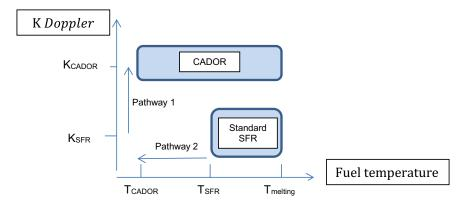
Fig. 3. CADOR operating domain compared to standard SFR.
