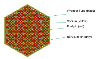
Fig. 4. CADOR fuel assembly (radial cut).
