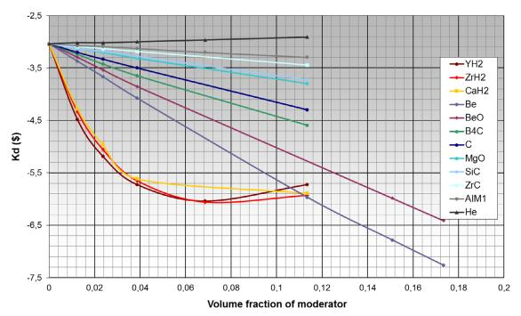
Fig. 1.  $K_{\text{Doppler}}$  for different types of moderators as a function of their core volume fraction.
