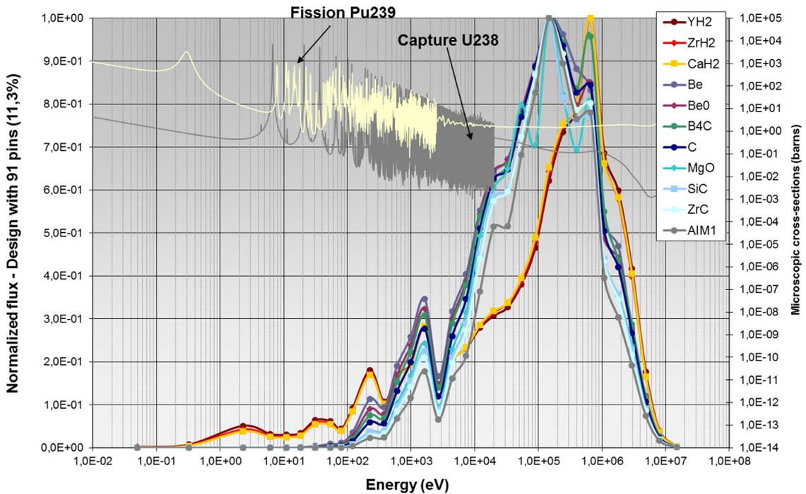
Fig. 2. Neutron spectra for different types of neutron moderator materials in the core (11% in volume fraction) compared with a reference case without moderator (AIM1).  $^{238}\text{U}$  capture and  $^{239}\text{Pu}$  fission cross sections are also plotted.
