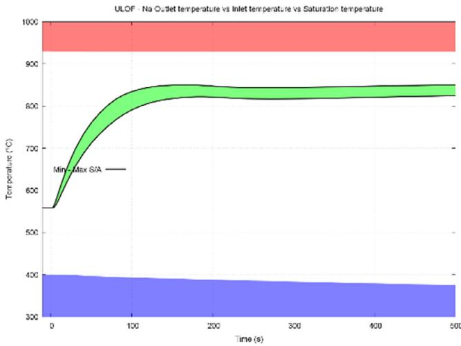
**Fig. 7.** Na outlet temperature.
