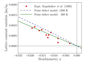
FIG. 4. Relative change in lattice constant as a function of x in  $UO_{2+x}$  for negative x (hypostoichiometric regime). The point defect model at 1200 K (dashed blue line) and at 300 K (solid green line) is compared to the XRD data from Ref. [1] (red circles).
