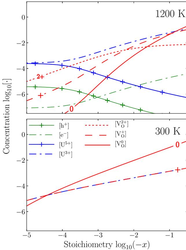
FIG. 3. Concentration per formula unit of the different species as a function of the stoichiometry of  $\text{UO}_{2+x}$  for negative  $x$  (hypostoichiometric regime) at 1200 K (upper panel) and at 300 K (lower panel). Only the dominant species are reported: delocalized holes and electrons (thin green lines), localized polarons (thick blue lines), and oxygen vacancies for different charge states (red lines).
