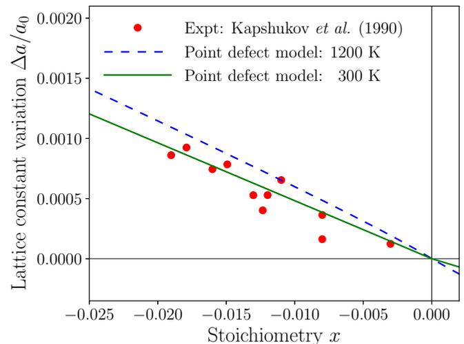
FIG. 4. Relative change in lattice constant as a function of  $x$  in  $\text{UO}_{2+x}$  for negative  $x$  (hypostoichiometric regime). The point defect model at 1200 K (dashed blue line) and at 300 K (solid green line) is compared to the XRD data from Ref. [1] (red circles).
