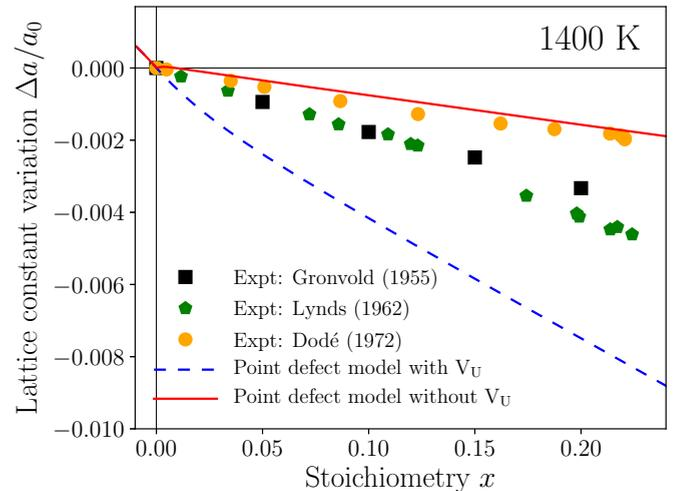
FIG. 6. Relative change in lattice constant as a function of  $x$  in  $\text{UO}_{2+x}$  for positive  $x$  (hyperstoichiometric regime) at 1400 K. The point defect models (lines) are compared to the high-temperature XRD data (symbols).
