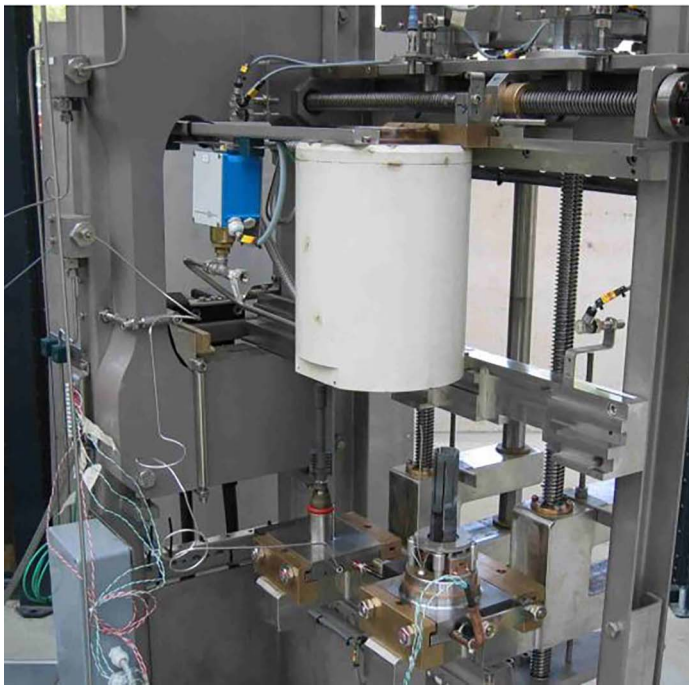
Fig. 1. The photo (left) and schematic view of the furnace (right).
