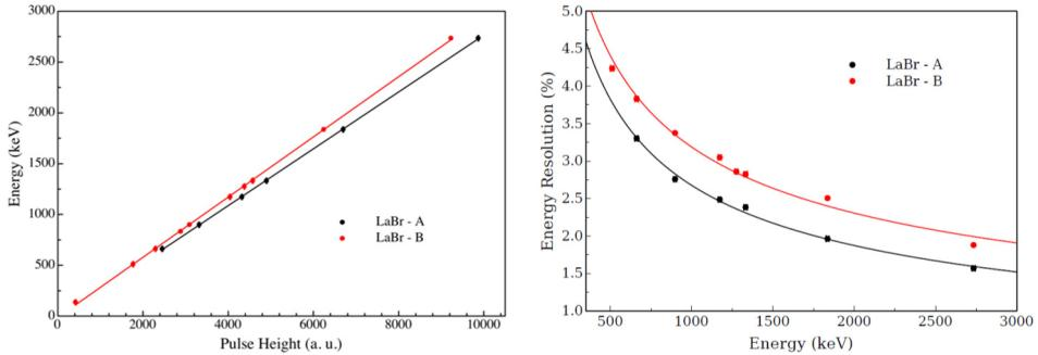
Fig. 5. (left) Energy calibrations and (right) energy resolution curves for the two 3 in  $\times$  3 in LaBr<sub>3</sub>:Ce scintillators.
