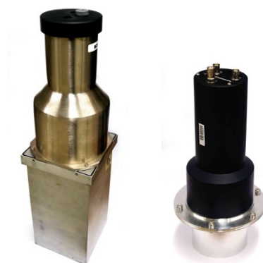
Fig. 2. View of NaI:Tl (left) and LaBr 3 :Ce (right) scintillators.
