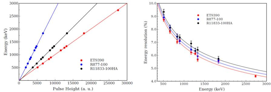
Fig. 3. (left) Energy calibration and (right) resolution curves for the three PMTs under study.
