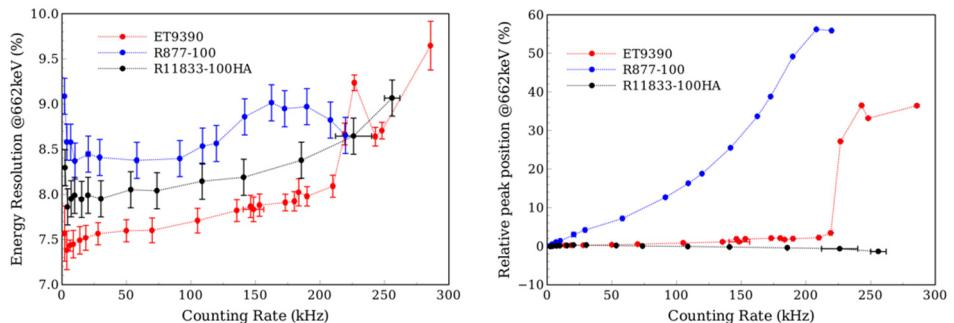
Fig. 4. (left) Energy resolution and (right) relative peak position at 662 keV as a function of the counting rate for the three PMTs under study.
