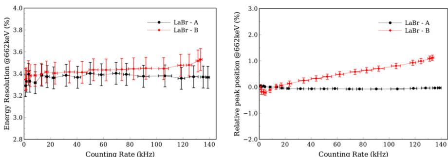
Fig. 6. (left) Energy resolution and (right) relative peak position at 662 keV as a function of the counting rate of the two 3 in  $\times$  3 in LaBr<sub>3</sub>:Ce scintillators.
