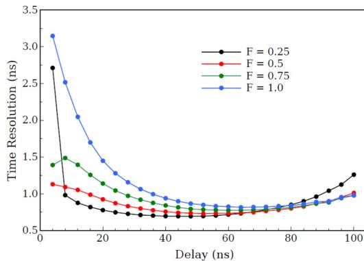
Fig. 7. Time resolution (FWHM) of the LaBr<sub>3</sub>:Ce system as a function of the DCFD delay for different values of fraction.
