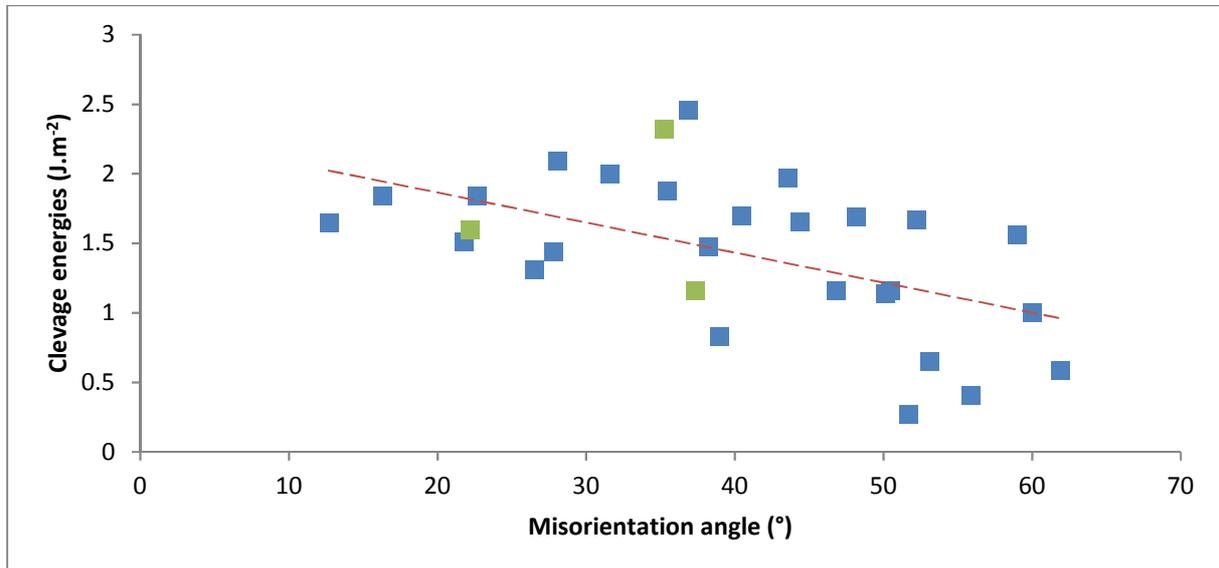
Figure 7. Misorientation dependence of the cleavage energies ( $\text{J}\cdot\text{m}^{-2}$ ) calculated with the Cooper potential for the 26 CSL grain boundaries (blue points) and the 3 semi-general grain boundaries (in green). The dashed line in red is the linear trend curve of the blue points.
