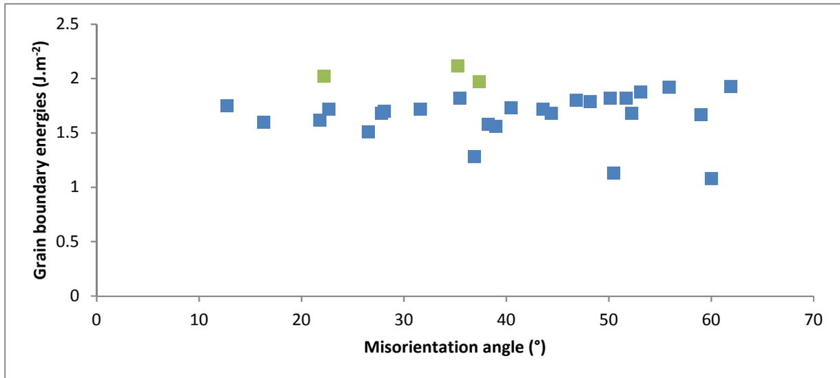
Figure 6. Misorientation dependence of formation energies ( $\text{J}\cdot\text{m}^{-2}$ ) for the 26 CSL grain boundaries (blue points) and the 3 semi-general grain boundaries (in green) calculated in this work with the Cooper potential.
