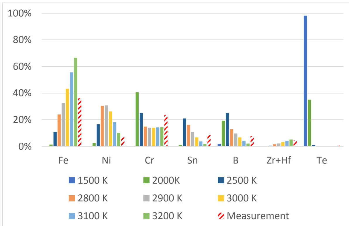
**Figure 5: Mass fractions of the major constituents of the aerosols: Calculations vs measurements**
