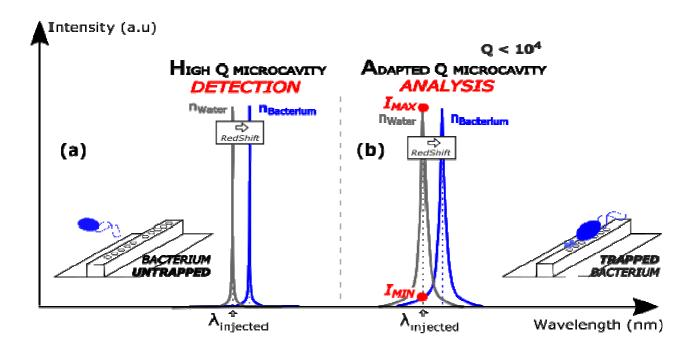
FIG. 1. Redshift of the microcavity resonance wavelength in presence of a bacterium above it.(a) High quality factor structure, ideal for detection of the target object, no trapping of bacteria.(b) Intermediate quality factor structure, ideal for bacteria trapping and analysis.
