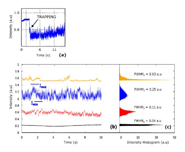
**FIG. 4. (a)** 20% drop in the optical signal transmitted by the microcavity, start of bacteria trapping. **(b)** Intensity transmitted by the microcavity during 10 seconds of trapping for the bacteria *S. epidermidis diplococcus* (orange), *E. coli* (blue), *B. subtilis aggregate* (red) and with no bacteria trapped (in bacteria and water medium) (black). **(c)** Histogram function of the transmitted optical signal.
