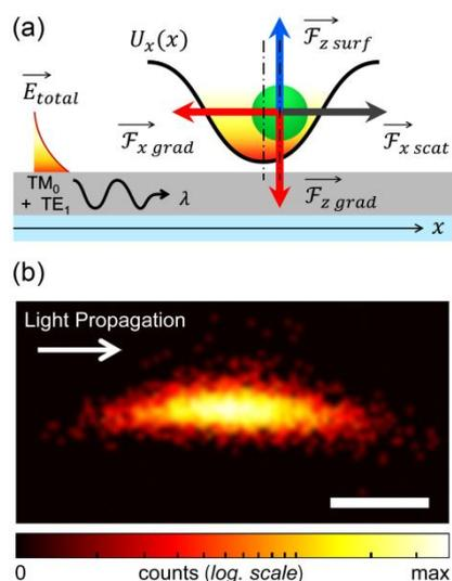
Fig. 4 Force equilibrium and trapping potential. (a) Schematic representation of the forces acting on a particle trapped in a TM<sub>0</sub>-TE<sub>1</sub> lattice. (b) Experimental map of the trapping potential experienced by a 1  $\mu\text{m}$  bead in a TM<sub>0</sub>-TE<sub>1</sub> lattice (scale bar: 250 nm).
