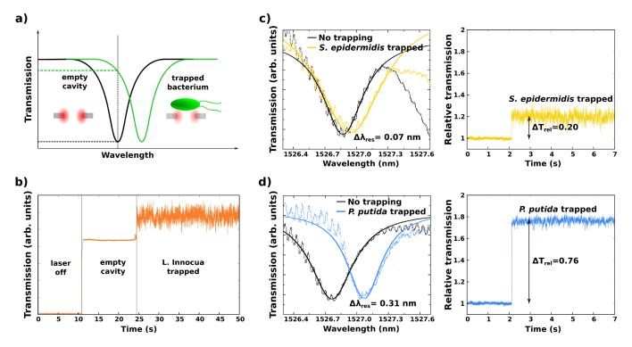
FIG. 2. (a) Representation of the redshift induced in the resonance frequency by a trapped bacterium. (b) Transmission recorded for *L. innocua*. (c) Minimum shift observed for *S. epidermidis* and minimum relative transmission augmentation. (d) Maximum shift observed for *P. putida* and maximum relative transmission increase.
