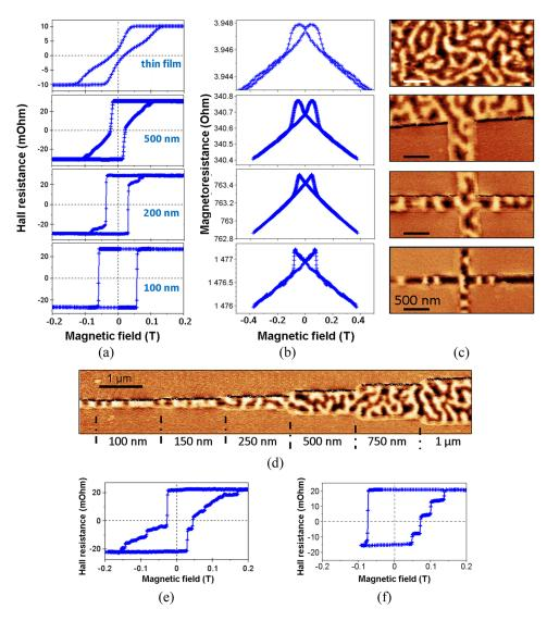
FIG. 3. a) EHE loops measured in the thin film and in crosses of various widths. b) Corresponding MR loops (measured with perpendicular magnetic field). c) MFM images of the corresponding structures in the as-grown magnetic state. d) MFM image of a structure consisting of wires of different widths, in the as-grown magnetic state. The nominal wire widths are indicated below the figure. e) EHE loop of a 200 nm wide cross at 10 K. f) EHE minor loop of a 100 nm wide cross at 10 K.
