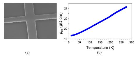
FIG. 2. a) Scanning electron microscopy image of a 500 nm wide cross (tilted sample). b) Temperature dependence of the longitudinal resistivity.
