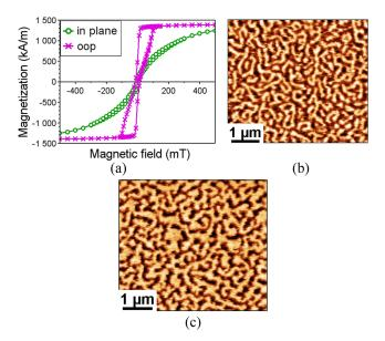
FIG. 1. a) In-plane and out-of-plane hysteresis loops at room temperature, measured using a SQUID magnetometer.  $5 \times 5 \mu m^2$  MFM image of the magnetic domains b) in an as-grown sample and c) in the remanent state after magnetic saturation.
