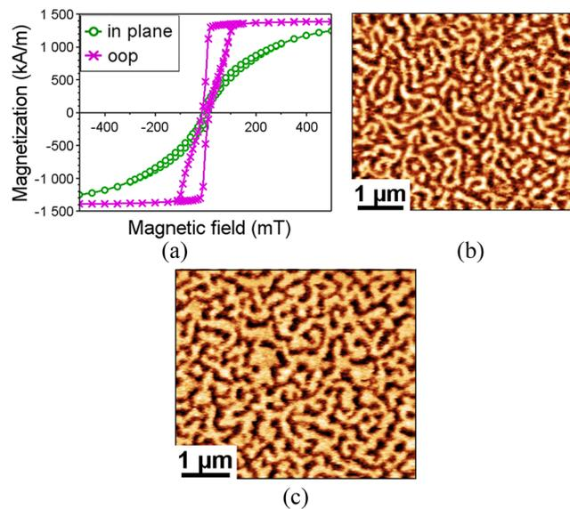
FIG. 1. a) In-plane and out-of-plane hysteresis loops at room temperature, measured using a SQUID magnetometer.  $5 \times 5 \mu\text{m}^2$  MFM image of the magnetic domains b) in an as-grown sample and c) in the remanent state after magnetic saturation.
