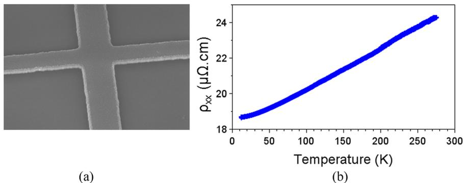
FIG. 2. a) Scanning electron microscopy image of a 500 nm wide cross (tilted sample). b) Temperature dependence of the longitudinal resistivity.
