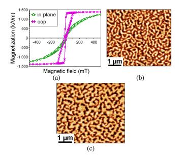
FIG. 1. a) In-plane and out-of-plane hysteresis loops at room temperature, measured using a SQUID magnetometer.  $5 \times 5 \,\mu m^2$  MFM image of the magnetic domains b) in an as-grown sample and c) in the remanent state after magnetic saturation.
