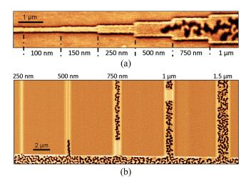
FIG. 4. a) MFM image of the structure consisting of wires of different widths, after saturation and partial magnetization reversal. b) MFM image of wires of different widths connected to a nucleation pad, after saturation and partial magnetization reversal.
