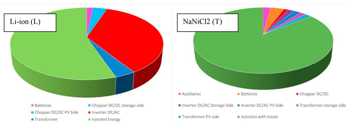
Figure 14. Energy balance of Li-ion (L) and NaNiCl<sub>2</sub> (T) power plants
