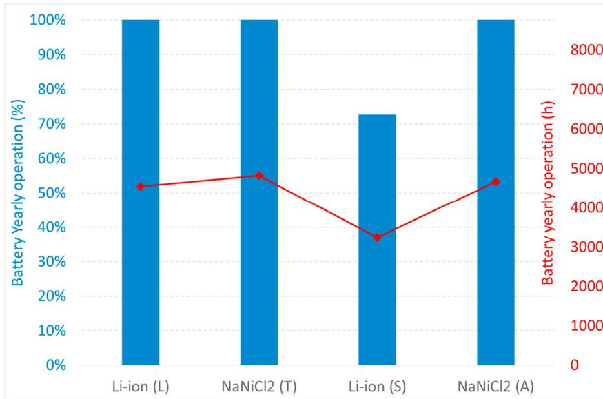
Figure 11. Battery yearly operation for 4 monitored ESS
