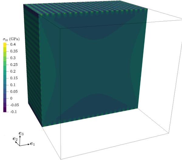
Figure 4: Stress component  $\sigma_{33}$  calculated by FE modelling of a macroscopic system. Surface tractions are set to the opposite of the tractions generated by the collection of loops inside the system (see for example Fig. 3-(a,d) for one of the surfaces). The macroscopic system contains  $21 \times 21 \times 21$  simulation boxes. Each box has a single prismatic loop in the middle (see text for details). The system is cut half-way along  $\mathbf{e}_2$  for the purpose of visualisation.
