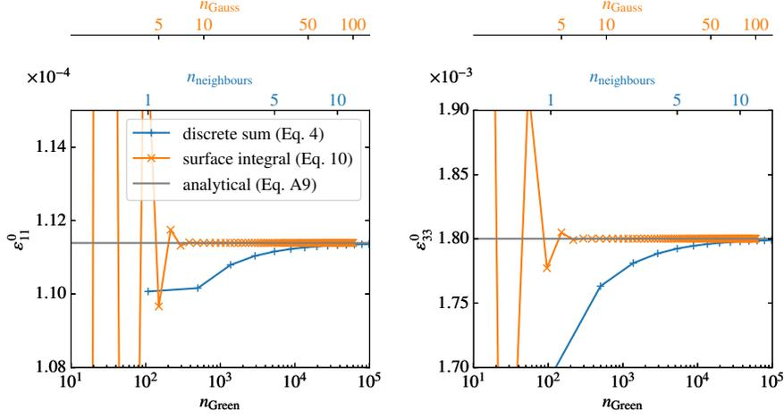
Figure 1: Comparison of the two approaches (discrete sum and surface integral) to evaluate the correction corresponding to a periodic elastic solution. The simulation box of edge length  $l = 10$  nm contains an interstitial prismatic dislocation loop of radius  $r = 2$  nm along  $x_3$  axis (see text for details). Two components are represented: (a)  $\varepsilon_{11}^0$  and (b)  $\varepsilon_{33}^0$ . The reference solution (Eq. (A.9)) is shown in gray.
