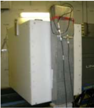
Fig. 10. Neutron detection block containing five 3 He detectors positioned against the neutron cell.
