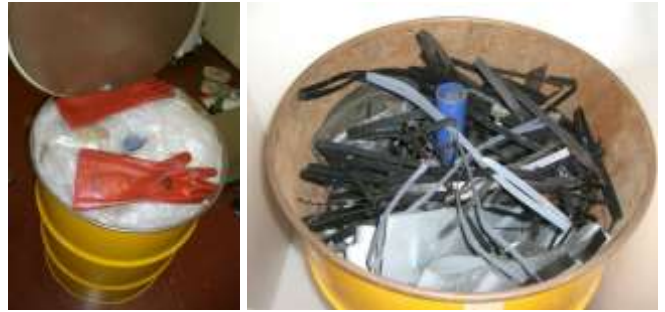
Fig. 15. Mock-up drums with central pipe allowing insertion of uranium samples. On the left: vinyl matrix of 0.02 \text{ g/cm}^3 average density. On the right: iron matrix of 0.22 \text{ g/cm}^3 average density.
