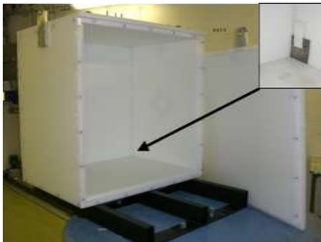
Fig. 8. Neutron interrogation cell (in open position) and foil position in irradiation setup No. 2.
