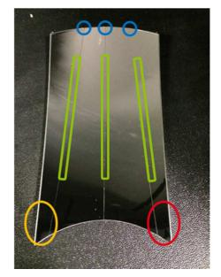
**FIGURE 8.** Picture of the mirror under test and locations of different singular points observed.
