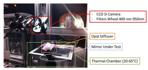
FIGURE 1. Experimental setup of the METHOD optimized for testing mirrors devoted to CPV systems.
