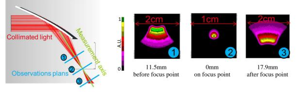
FIGURE 5. Schematic configuration of the mirror, the measurement axis and the observation plans with TracePro Modelling. **FIGURE 6.** Spot diagram of the focused light along the measurement axis for three observation plans, situated before, on and after the focus point.
