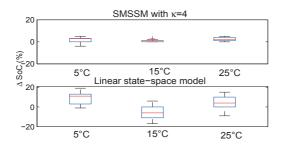
Fig. 4. Boxplots of  $\Delta SoC = SoC(Ah-counting) - SoC(SMSSM)$  with  $\kappa = 4$  (top) and Linear state-space model (bottom) for ambient temperature equal to 5, 15, 25°C
