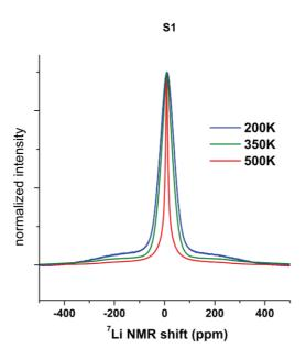
**Fig. S2**: Experimental <sup>7</sup>Li NMR spectra of S1 sample at different temperatures. The spectra are deconvoluted by combining a narrow central line (central transition) and a wider contribution (satellite transitions) with lower intensity.
