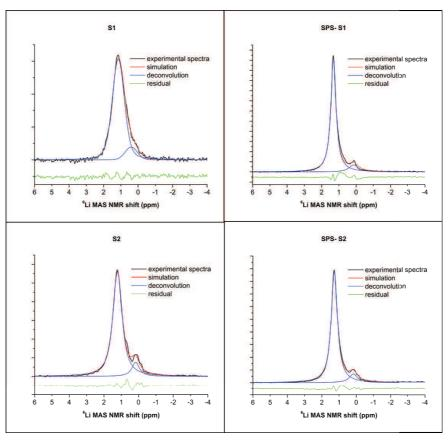
**Fig. S3**: Experimental and simulated <sup>6</sup>Li MAS NMR spectra of the studied samples at room temperature.
