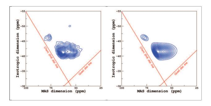
**Fig. S6:** Experimental (left) and simulated (right) <sup>27</sup>Al MQMAS spectra of S2.
