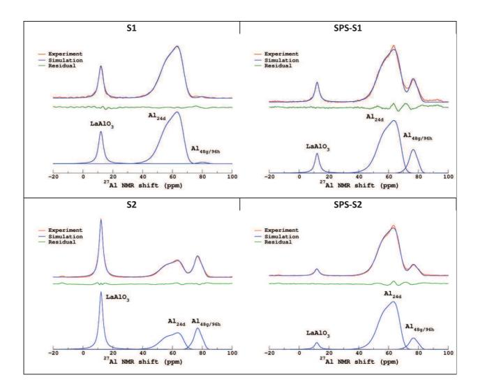
**Fig. S4**: Experimental and simulated <sup>27</sup>Al MAS NMR spectra of studied samples at room temperature.
