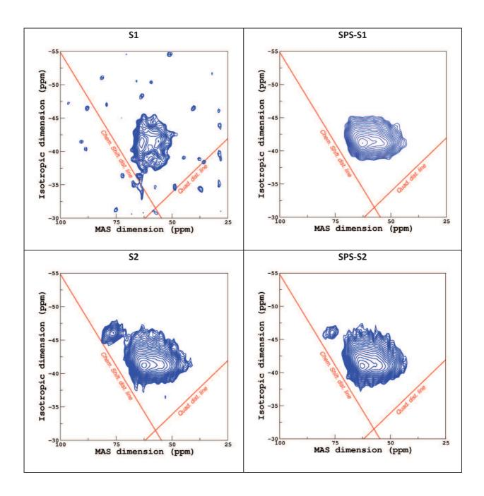
**Fig. S5**: Experimental <sup>27</sup>Al MQMAS NMR spectra of the studied samples at room temperature.
